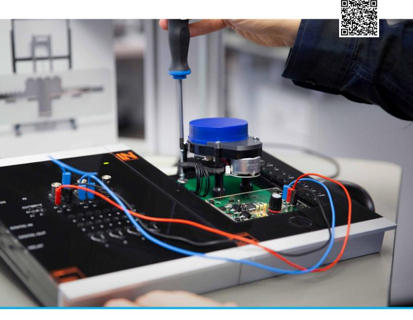
A direct introduction to the topic of LIDAR (Light Detection and Ranging): Use this training system to teach industry level diagnostic skills that include optical distance and speed measurement. The hardware of this driver assistance teaching system is based on a real, industry standard LIDAR module, giving trainees valuable insights into how the system works on a real vehicle.
