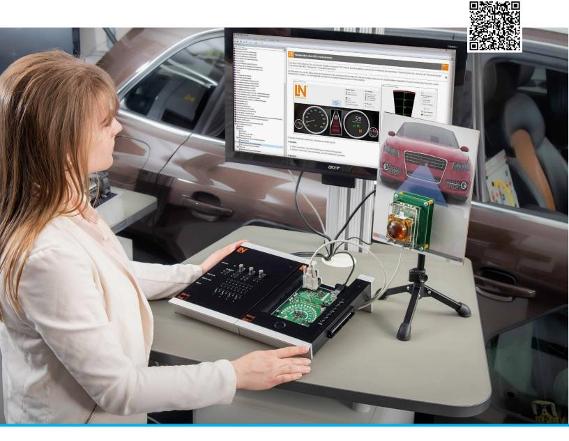
This UniTrain course introduces the trainee to the fundamentals of adaptive cruise control (ACC) including the emergency brake assistant. In addition to setting up and networking the system, all the individual components that make up the driver assistance system are discussed in detail. A major focus is placed on the calibration of the radar sensor. This is carried out using a hands on calibration target. The module can then be optimally aligned using the adjustment points on the ACC module.
