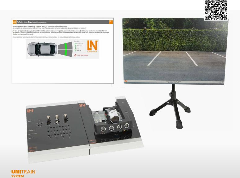
Another driver assistance system that's important in assisting large SUVs or sedans in narrow parking spaces. Our UniTrain course includes a complete backup system for a vehicle using several ultrasonic sensors and a reversing camera. Trainees gain real world practical skills into the handling and diagnosis of the system. This enables them to learn about the physical limitations of the assistance system along with ways to troubleshoot different malfunctions.
