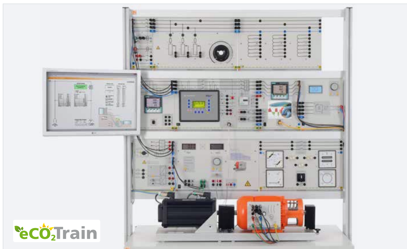
Example experiment "Smart grid supplement to ESG 1: Pumped-storage hydroelectric plant EUG 3"
