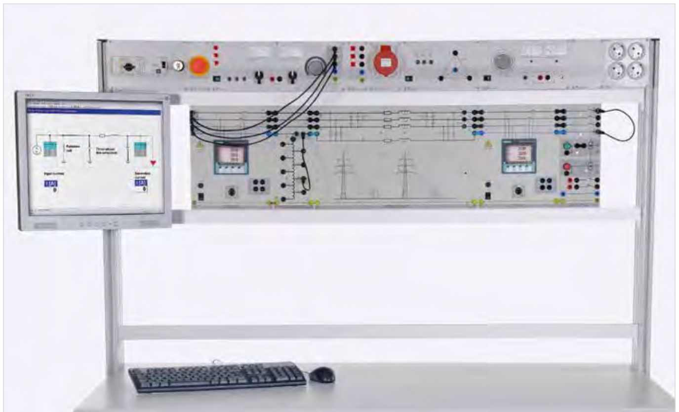
Sample experiment "Investigations on lines with earth-fault compensation" EUL 3
