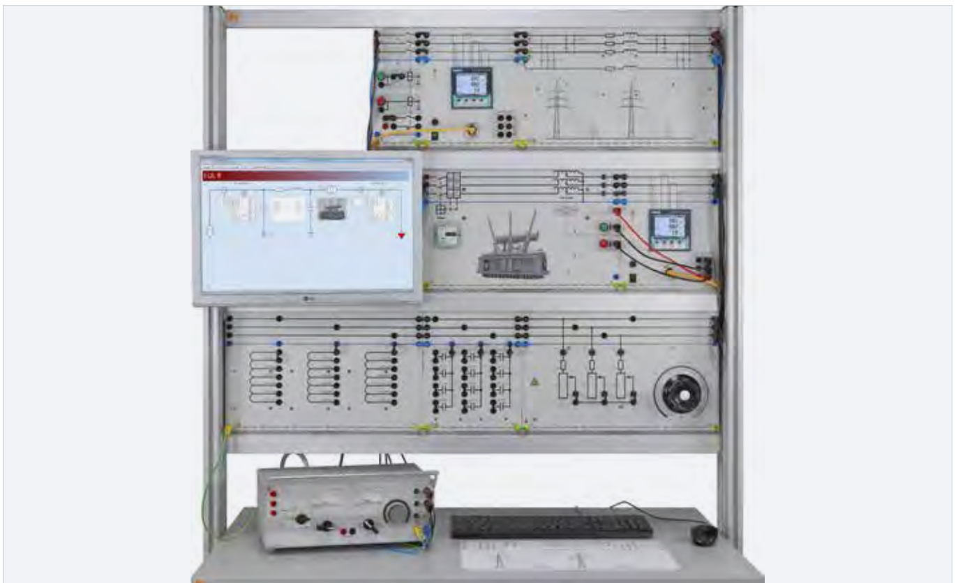
Experiment example "Load-dependent voltage control of a power line EUL8"
