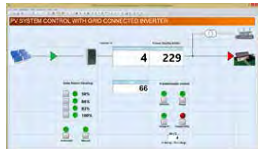
SCADA with derating of photovoltaic inverter
