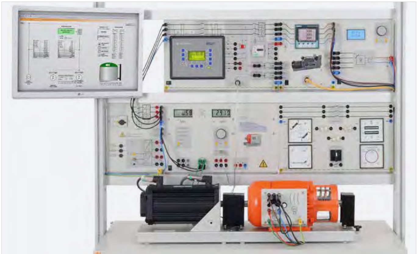
Sample experiment "Automatic synchronising circuits" EUG 2
