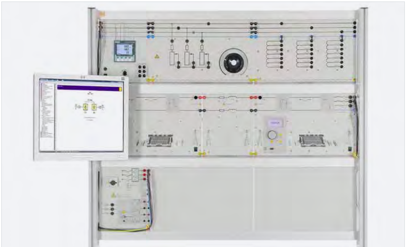
Experiment example "High voltage DC transmission" EDC1
