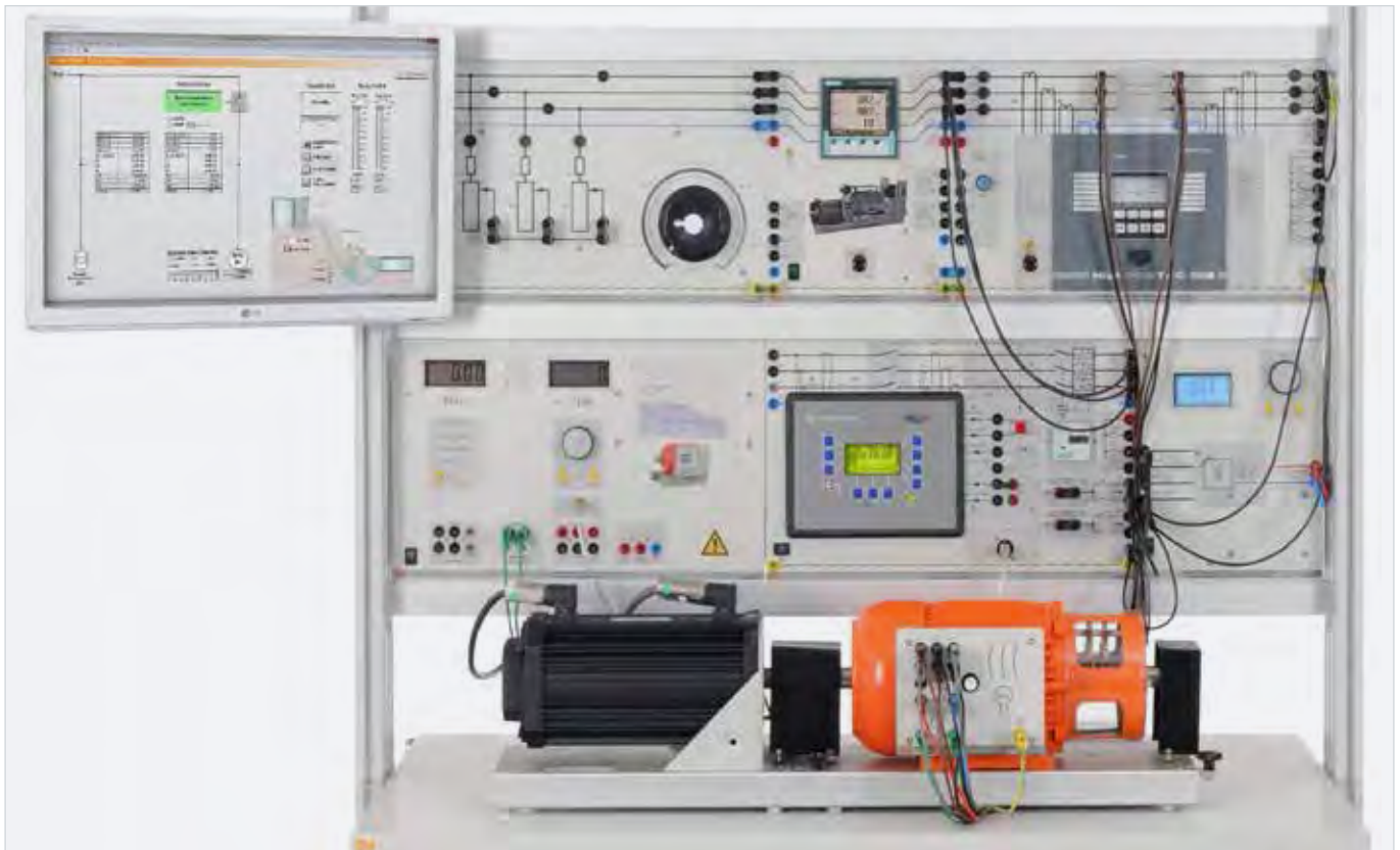
"Generator differential protection" EGP 2
