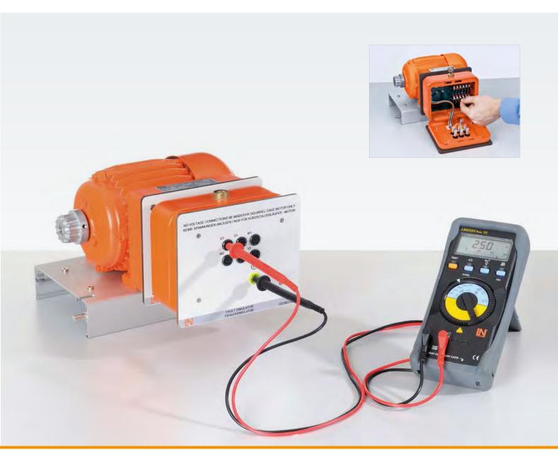
The fault simulator can be simply plugged into a three-phase asynchronous machine. Thanks to the lockable fault switches, a wide variety of typical faults can be activated. These can be found and analyzed using measuring equipment routinely found in industrial applications. Repair strategies can be derived based on the measurement results. All measurements are undertaken with the equipment de-energized.
