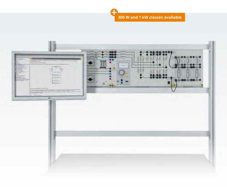
Line-commutated converters permit power to be fed from an AC or three-phase system to a DC circuit. These can be designed for operation in controlled mode using thyristors and triacs or uncontrolled mode using diodes.
