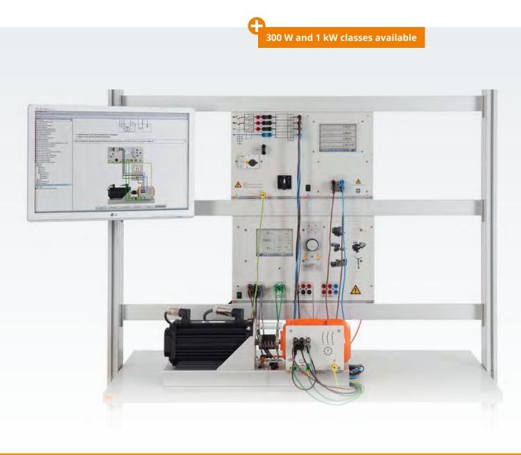
Reluctance motors are a mixture of asynchronous and synchronous motor. Thanks to the special rotor design with salient poles, the motor can start like an asynchronous motor. After a certain speed is reached, the rotor runs synchronously with the stator field. Reluctance machines are used for example in the textile industry for the synchronous de-spooling of yarn. This entails several motors being controlled by one frequency converter.
