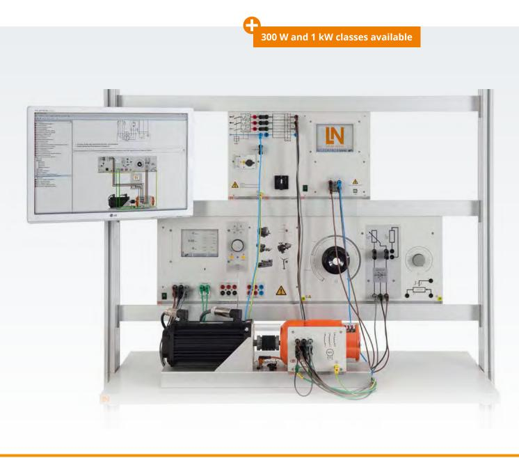
In contrast to squirrel-cage rotors, slip-ring rotors have a rotor equipped with wound coils. These can be connected to resistors or static converters via slip-rings. Speed adjustment is performed via these connection terminals.
