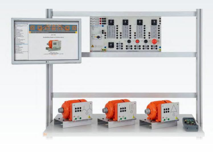
The focus of this training section is the development of circuitry and the correct selection of switching elements and devices. Multi-pole motors can be connected up to a certain power class directly in the three-phase circuit. To do this, there is the appropriate switching equipment for every application and purpose.
