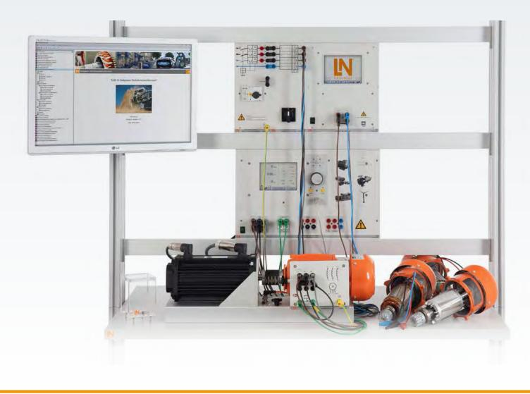
This training system comprises one uniform stator for all machine types and a set of interchangeable rotors. Thanks to its dismountable design, this set is particularly well suited for teaching fundamentals because it facilitates the exploration of the construction designs and differences between the various machines.
