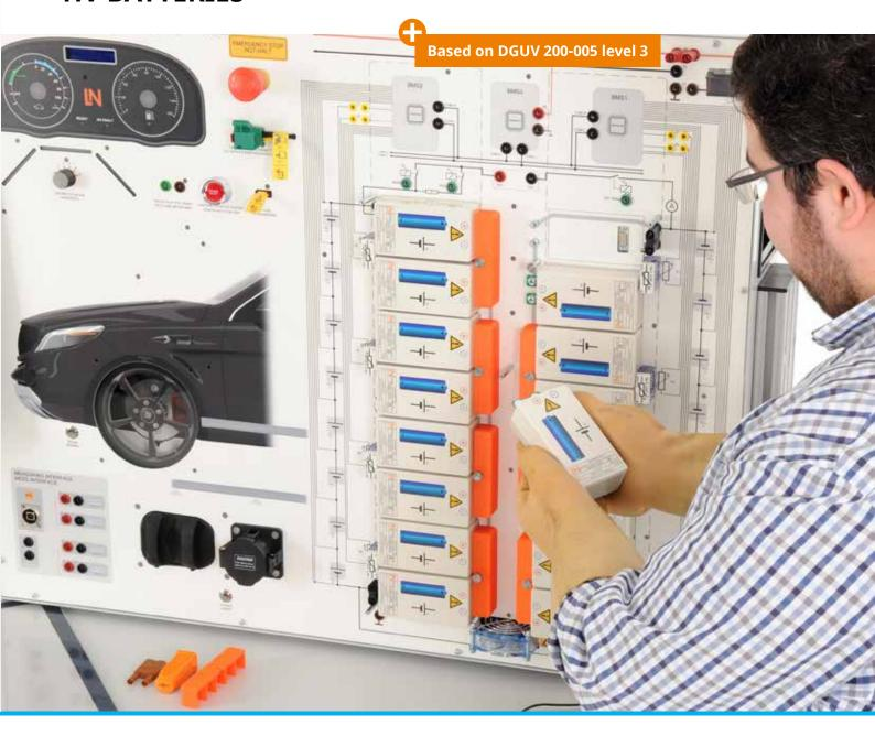
Working directly on a real high-voltage battery and inside it: The system is set up to be just like a high-voltage battery in a standard production vehicle. With this training system, trainees can make measurements and diagnoses inside the high-voltage battery, working down to the level of individual cells and even replacing them.
