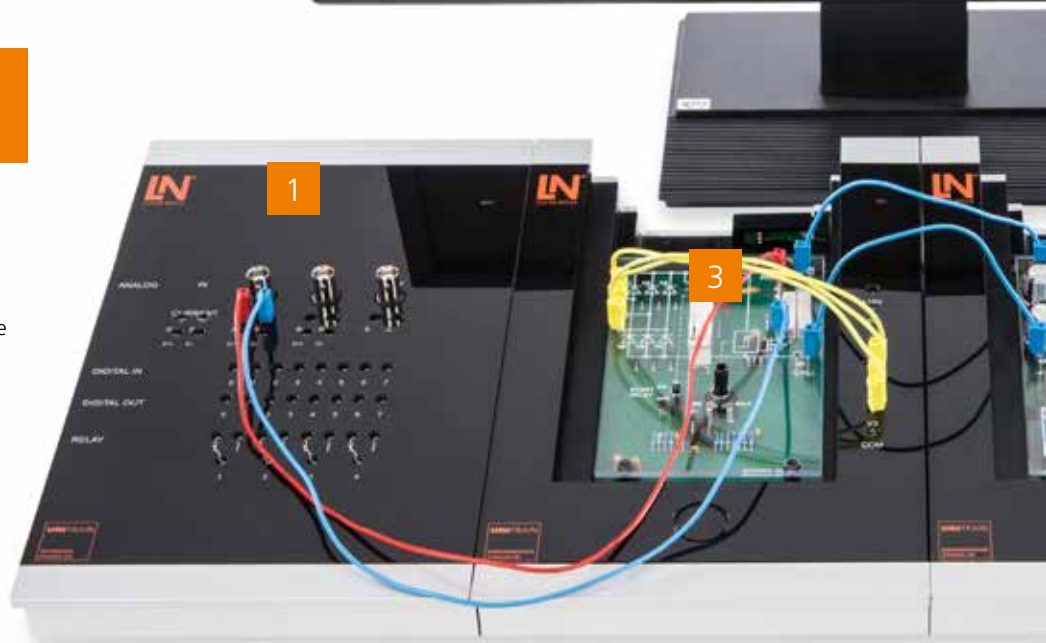
1 UniTrain interface Measurement and control interface: Analog / digital measurement inputs and voltage sources for experiments
