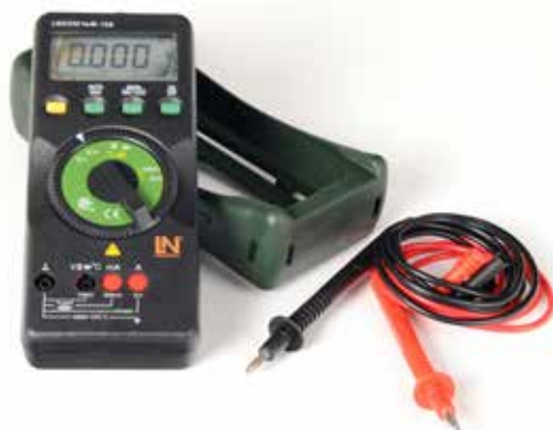
Multimeter with optical data interface for display via a virtual instrument on a PC
