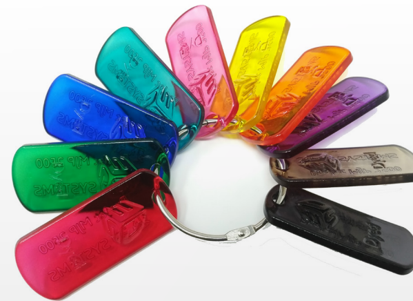
Visijet M2R-CL color keyring with clear coating dyed with standard colors with 1% concentration (60 °C and 30 min)
