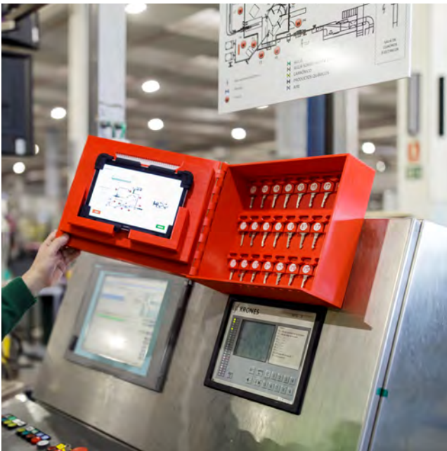
Red material not only increases visibility, but can also increase awareness of 3D printing in use on the plant floor
