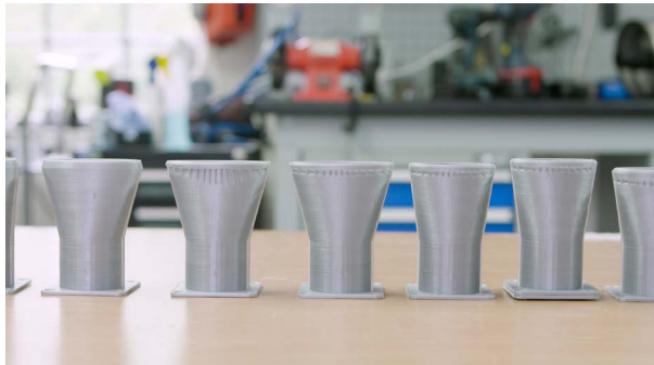
Iterations of the complex nozzle design (L) and the final 3D printed part in action (R)
