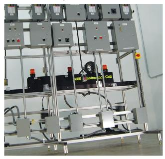
The construction of the cell can be performed entirely by the trainees. Using industry-standard work orders, standard operating procedures, schematic diagrams and technical manuals as resources, students assemble the components and install the electrical wiring and controls for the cell and add-on components.
