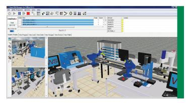
OpenCIM Offline is the simulation version of OpenCIM. Users can design and run an unlimited variety of CIM or FMS cells in simulation mode.
