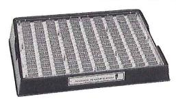
The15200 Circuit Panel has150 phosphor bronze contact islands enclosed in clear plastic. Each island matches five holes through the top surface for insertion of mounted and unmounted components and standard hook-up wire. The ECI circuit panel provides 750 contacts and measures 14-11/16 L x 9-5/8 W x 1/2 T.
