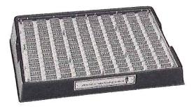
The 15200 Circuit Panel has150 phosphor bronze contact islands enclosed in clear plastic. Each isl and matches five holes through the top surface for insertion of mounted and unmounted components and standard hook-up wire. The ECI circuit panel provides 750 contacts and measures 14-11/16" L x 9-5/8" W x 1/2" T.
