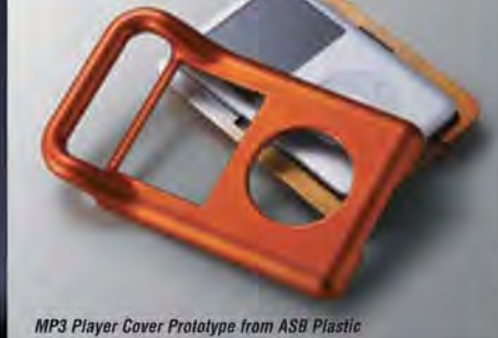
MP3 Player Cover Prototype from ABS Plastic
