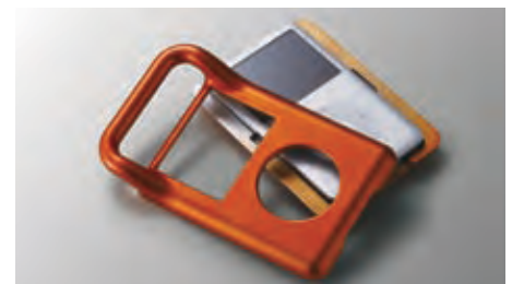
ABS iPod prototype case milled with SRP.
