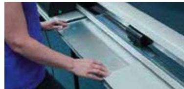
PowerTech cuts up to 3mm flexible substrates
