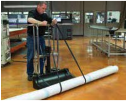
1. Nylon safety straps allow solo users to pull media rolls into the securing tray for transport.
