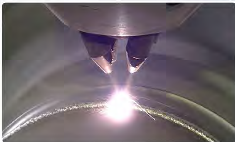
LENS in action repairing a casing
