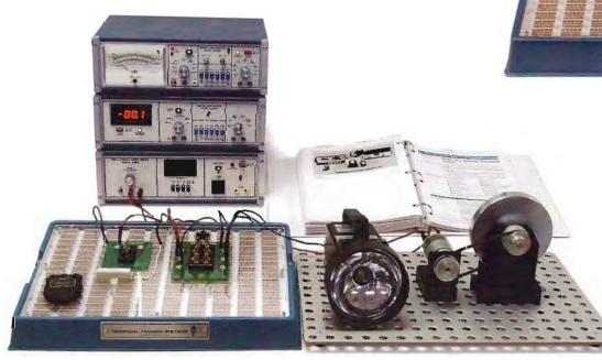
Using the equipment shown, students determine the mechanical power stored in a flywheel system.
