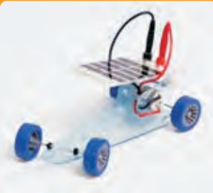
▲ Auto chassis with solar module
