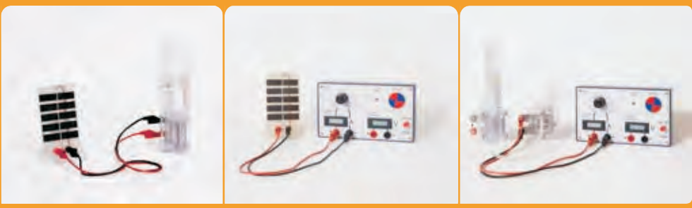
▲ Solar module with electrolyzer
