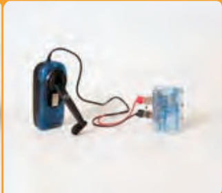
▲ Hand generator with reversible fuel cell
