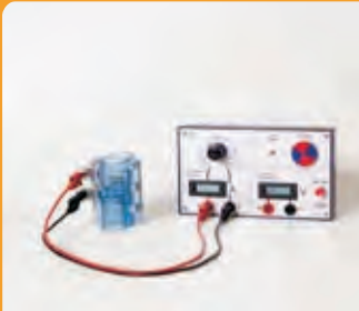
▲ Reversible fuel cell with load measurement box
